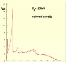
Figure 3: Calculated coherent intensity for  $E_0=120$  MeV. No beam divergence and straggling in radiator is considered.
